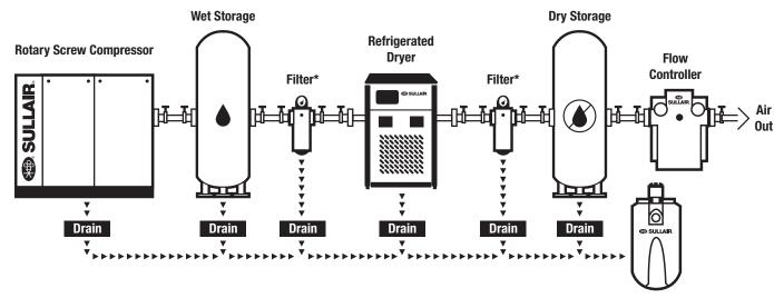
\* Models RFA-10 through RFA-1600 include integrated filters. Models RFA-2000 through RFA-7300 require a pre- and after-filter as shown.
